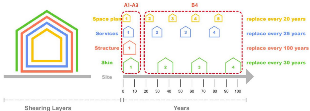
Figure 2. Shearing Layers and assumed life spans. Source: Author's own image based on Brand (1994) and Dodd & Donatello (2020)
